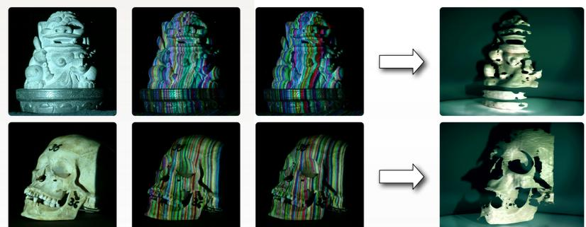
Three input images (a plain white and two structured light projections) are required for each of the above reconstructions.
