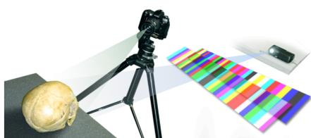
Our minimalistic projector-camera based 3D scanner uses a time-coded color structured light.
