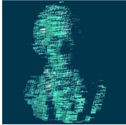
Figure 4.14: Triangulated point cloud with plane background masking and artifact elimination through meshing threshold=0.4 with illuminated triangles.
