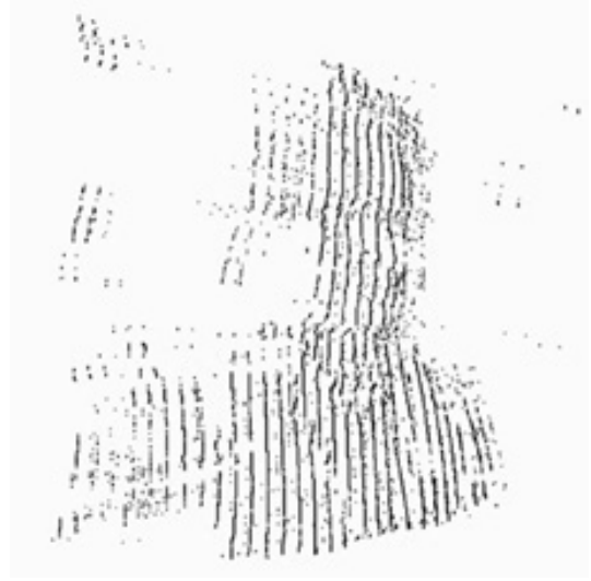
Figure 4.10: Triangulated point cloud without plane background masking and artifact elimination through meshing threshold=0.4.
