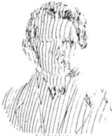
Figure 4.3: Edge detection without consecutive edge pixel restriction and threshold=0.002.
