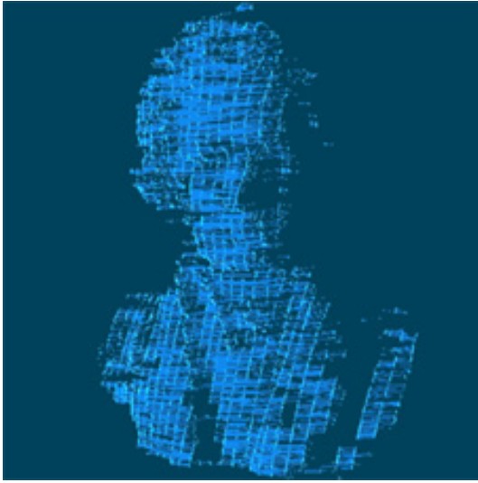
Figure 4.13: Triangulated point cloud with plane background masking and artifact elimination through meshing threshold=0.4 with meshed triangle surfaces.
