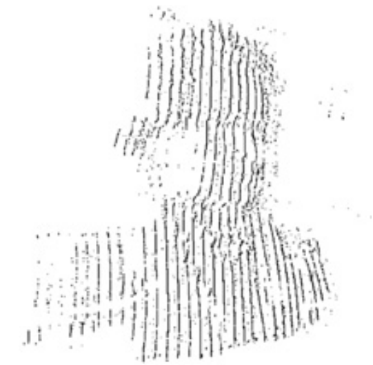
Figure 4.12: Triangulated point cloud with plane background masking and artifact elimination through meshing threshold=0.4.
