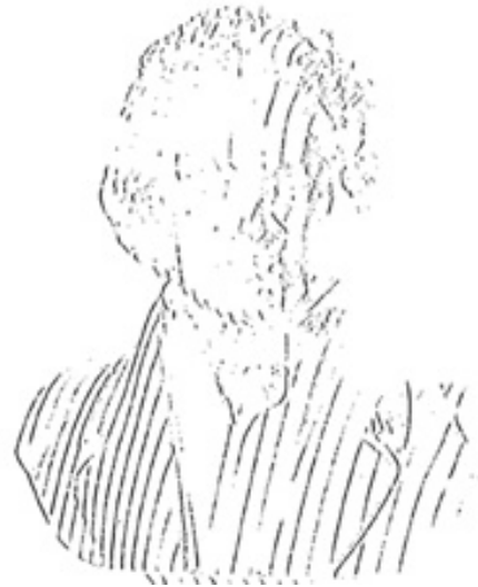
Figure 4.6: Edge detection with restricting 10 consecutive edge pixels and threshold=0.002.
