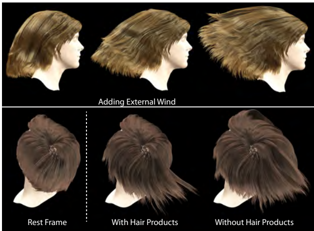
Figure 18: After acquiring parameters we can simulate with additional external forces, and the simulated hair will remain faithful to the captured actor. The top row shows three animation frames from one actor with strong wind. The bottom row shows that the same wind force applied to the short-haired actor with and without hair product gives very different (and expected) behavior.
