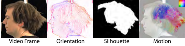
Figure 5: Our optimization will use cues from the video frames. The constraints include the 2D orientation of strands, the silhouette of the hairstyle volume, and approximate motion vectors.
