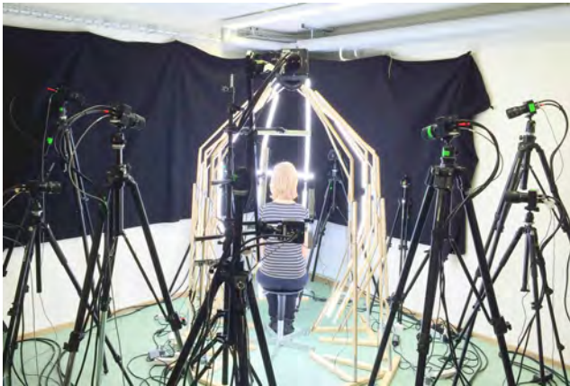
Figure 3: Our capture setup consists of 8 video cameras spaced evenly around the hairstyle, and 2 additional cameras tracking head motion from front. The hair is uniformly lit using LED strips.
