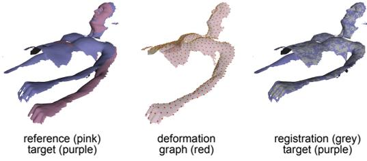
**Figure 2:** Graph-based non rigid ICP for surface tracking.
