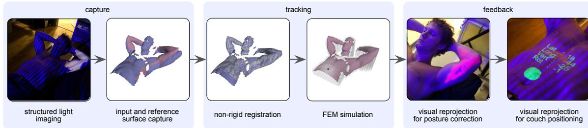
**Figure 1:** Our pipeline begins with a real-time structured light-based surface capture. The tumor position is then tracked using a non-rigid registration and FEM simulation framework. Finally, visual guidance is projected onto the patient for accurate posture correction and couch positioning. Notice that the reference surface can either be the initial frame or a full CT capture.
