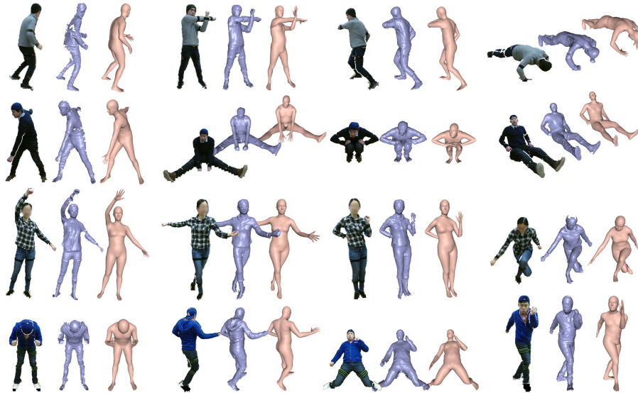
Fig. 5. Example results reconstructed by our system. In each grid, the left image is the color reference; the middle one is the fused surface geometry; and the right one is the inner body shape estimated by our system.
