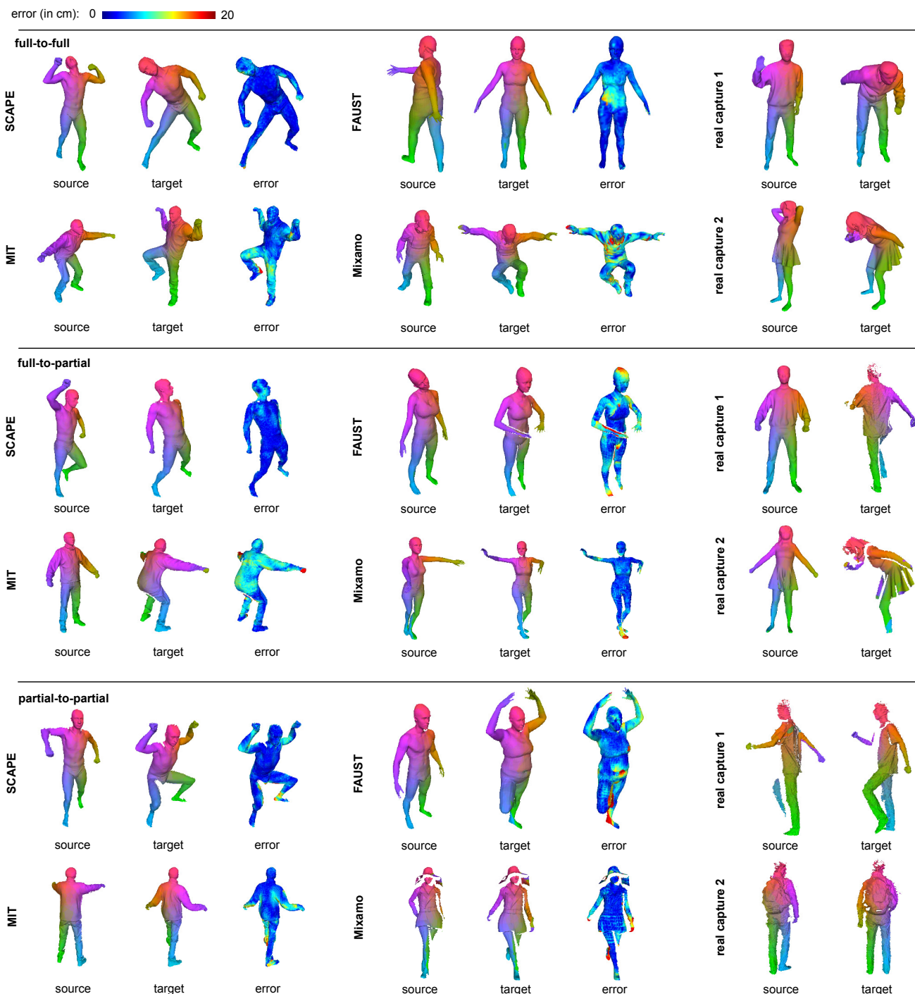
Figure 5: Our system can handle full-to-full, partial-to-full, and partial-to-partial matchings between full 3D models and partial scans generated from a single depth map. We evaluate our method on various real and synthetic datasets. In addition to correspondence colorizations for the source and target, we visualize the error relative to the synthetic ground truth.
