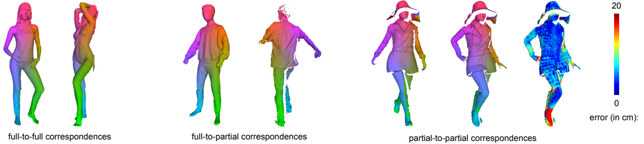
Figure 1: We introduce a deep learning framework for computing dense correspondences between human shapes in arbitrary, complex poses, and wearing varying clothing. Our approach can handle full 3D models as well as partial scans generated from a single depth map. The source and target shapes do not need to be the same subject, as highlighted in the left pair.
