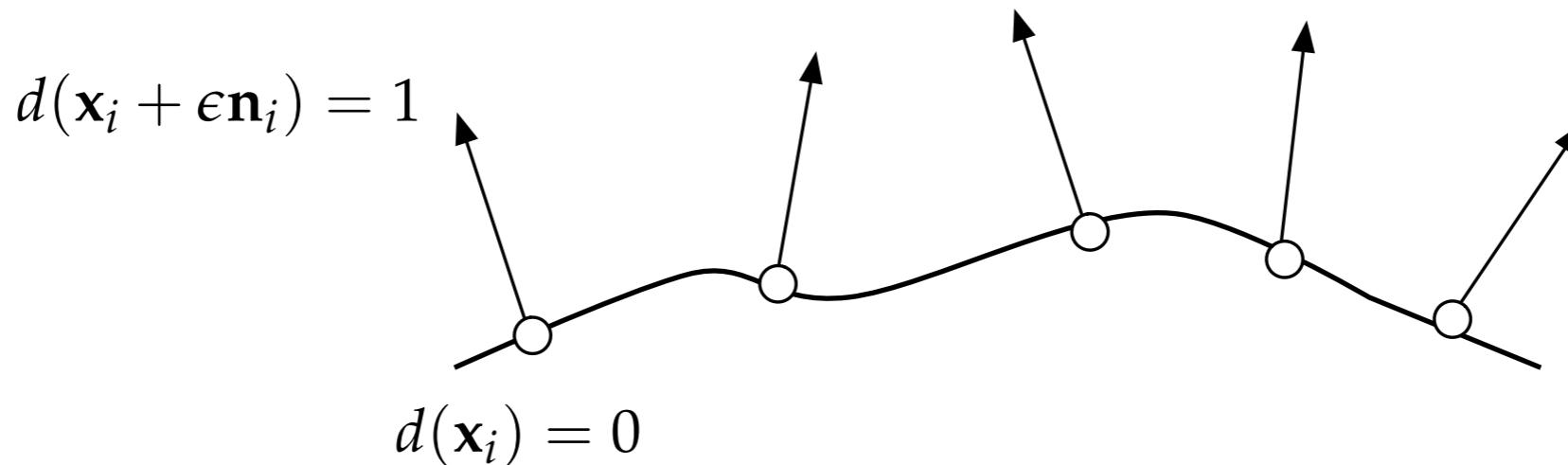
$$\begin{bmatrix} \phi(\|\mathbf{x}_1 - \mathbf{x}_1\|) & \dots & \phi(\|\mathbf{x}_1 - (\mathbf{x}_n + \epsilon \mathbf{n}_n)\|) \\ \vdots & \ddots & \vdots \\ \phi(\|(\mathbf{x}_n + \epsilon \mathbf{n}_n) - \mathbf{x}_1\|) & \dots & \phi(\|(\mathbf{x}_n + \epsilon \mathbf{n}_n) - (\mathbf{x}_n + \epsilon \mathbf{n}_n)\|) \end{bmatrix} \begin{bmatrix} w_1 \\ \vdots \\ w_{2n} \end{bmatrix} = \begin{bmatrix} d_1 \\ \vdots \\ d_{2n} \end{bmatrix}$$
