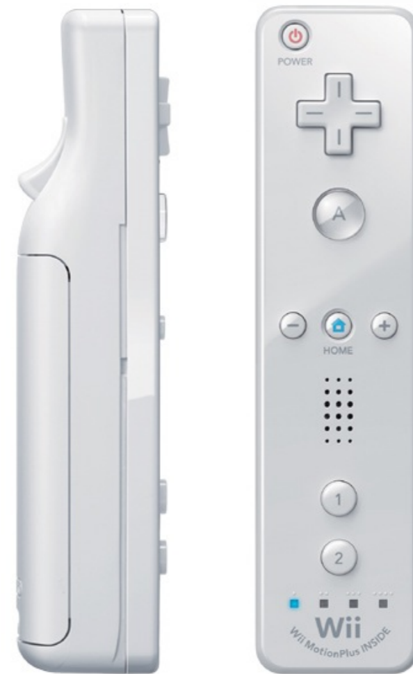
Wii remote Accelerometers, IR sensor
